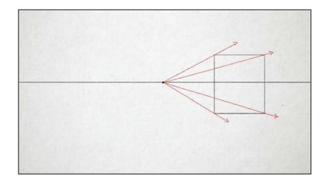
Using these lines as a guide, we'll draw a second rectangle. Each corner of the second, smaller rectangle should touch each of the four receding lines.
