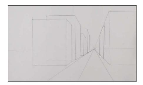
We can easily add a curb for our sidewalk by adding a couple of lines that recede back to the vanishing point. Cracks in the sidewalk are added by drawing horizontal lines that get closer together as they extend back in space.
