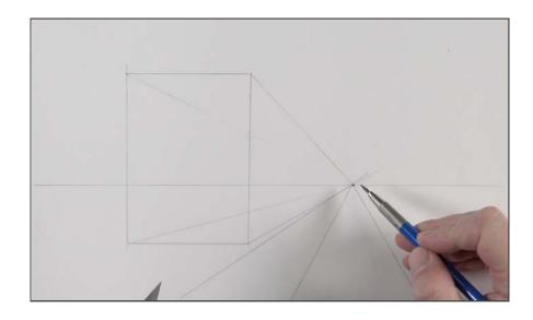
After adding a vertical line for the back end of the building, we can erase the lines that are no longer needed. Now we have our first form in place. We'll add details in a moment, after we have all of the forms in place.
