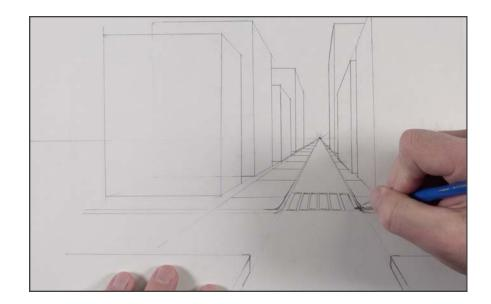
We can add as many details as we like. Windows, doors, and signs on the sides of the buildings are added by using lines that go back to the vanishing point. The vertical edge of each window or door is simply a vertical line.
